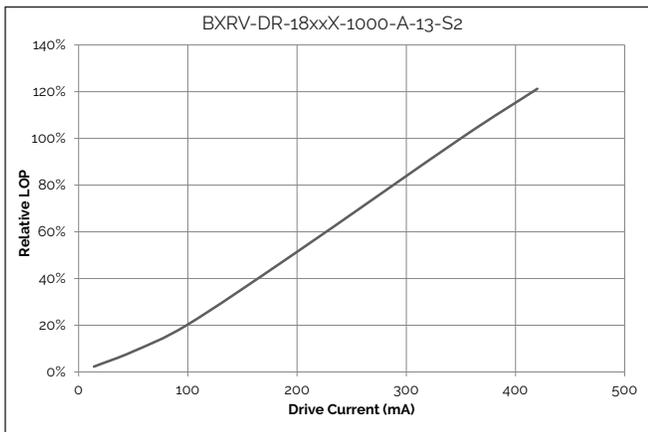
**Figure 13: 12W Relative LOP vs. Drive Current,  $T_c=25^\circ\text{C}$**
