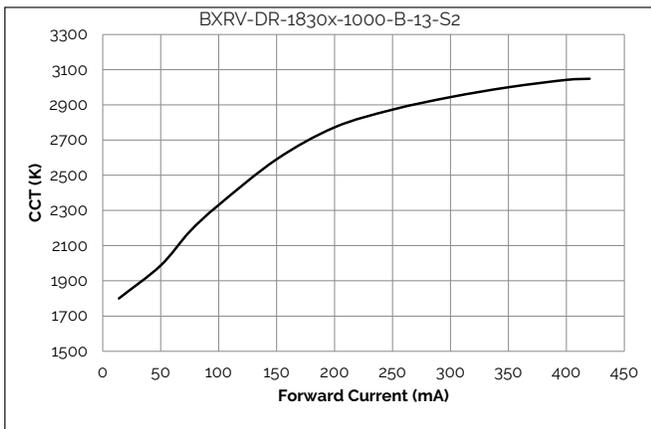
**Figure 10: 12W CCT vs. Forward Current,  $T_c=25^\circ\text{C}$**
