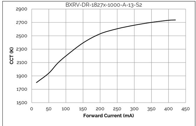
**Figure 9: 12W CCT vs. Forward Current,  $T_c=25^\circ\text{C}$**
