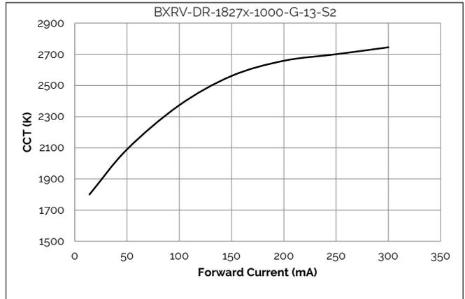
**Figure 7: 6W CCT vs. Forward Current,  $T_c=25^\circ\text{C}$**
