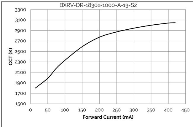
**Figure 8: 6W CCT vs. Forward Current,  $T_c=25^\circ\text{C}$**
