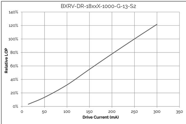
**Figure 12: 6W Relative LOP vs. Drive Current,  $T_c=25^\circ\text{C}$**
