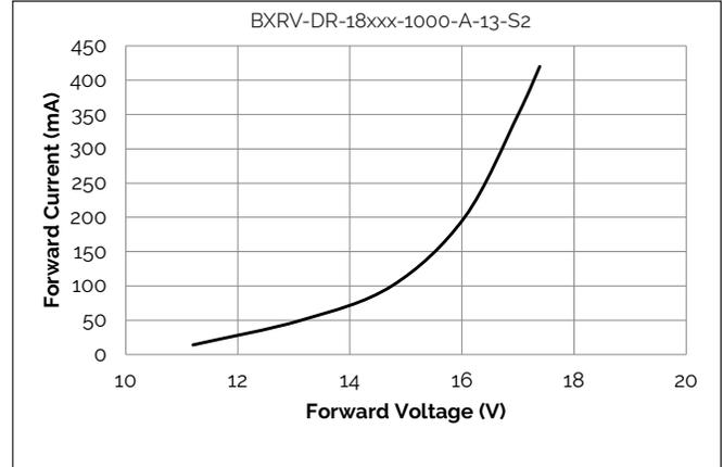
**Figure 3: 12W Forward Voltage vs. Forward Current,  $T_c = 25^\circ\text{C}$**
