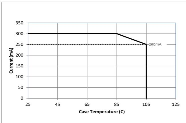
**Figure 17: Derating Curve 6W, 12W**
