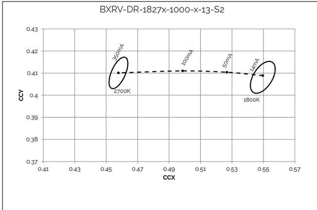
**Figure 15: Color shift vs. Forward Current 3000K - 1800K**
