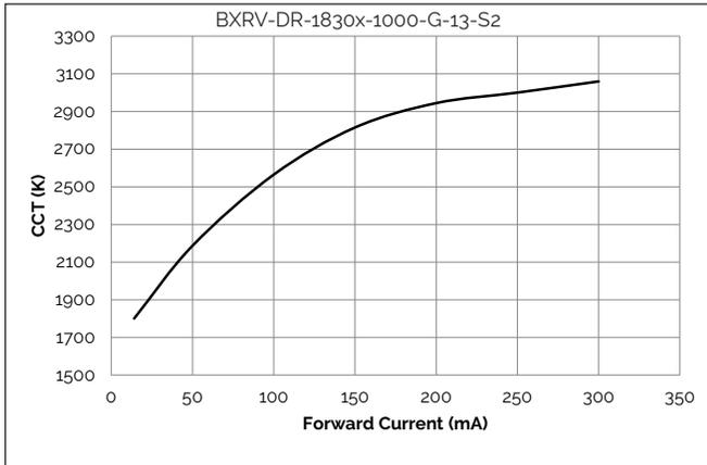
**Figure 6: 4W CCT vs. Forward Current,  $T_c=25^\circ\text{C}$**
